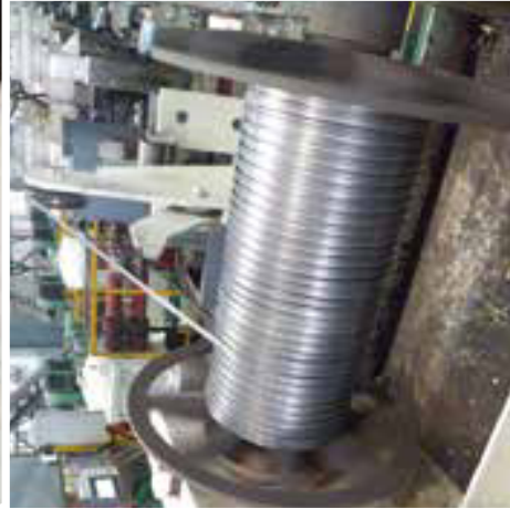
▲ 套筒加工 Continuous rolling of bush material
